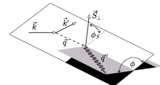
$$A_{UL} = \frac{N_{s_z=+} - N_{s_z=-}}{N_{s_z=+} + N_{s_z=-}} = \frac{\sqrt{\epsilon(\epsilon+1)} \sin \phi F_{UL}^{\sin \phi}}{F_{UU,T} + \epsilon F_{UU,L}} + \frac{\epsilon \sin 2\phi F_{UL}^{\sin 2\phi}}{F_{UU,T} + \epsilon F_{UU,L}}$$
