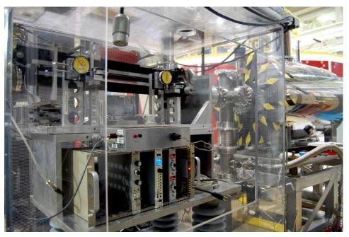
Transformer Translation Stage Sensor? Bertran HV Supply DVM (30ish kV) Optical Transmitte GPIB Optical 30-ish kV Floating Platform Insulating supports Grounded Cage With Access and Interlocks Optical GPIB Optical on Access Reciever Front Rue 50 Din Dibbon
