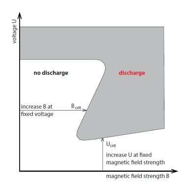
The instability of these systems depends on the magnetron orbits of ions and critical ionization energy of the residual gasses. It is not well studied and geometry dependent.
