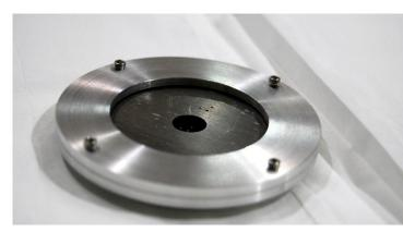
Precision machined Cadmium mask for Dy foil in collimator mount.
