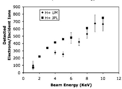
FIG. 9. The response of the delta-doped CCD to H<sup>+</sup> beam. The squares represent the data obtained by JPL in 1999 using the CCD in imaging mode to detect individual protons (Ref. 13). The diamonds represent our data obtained in this study using the CCD in current mode.
