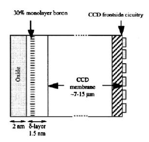
FIG. 5. Schematic of delta-doped CCD structure (not to scale) showing boron atoms 0.5 nm below the silicon epilayer surface and protected by an oxide overlayer. Delta-doped CCDs are back-illuminated devices, meaning that particles are incident on the back surface. [Adapted from Nikzad *et al.* (Ref. 13).]
