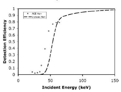
FIG. 4. Solid-state detector efficiencies for He<sup>+</sup> for the ACE and Ulysses spacecraft. Improved technology for the ACE mission allows He<sup>+</sup> to be detected at lower energies compared to the Ulysses SSD. However, ions below 25 keV still elude detection.
