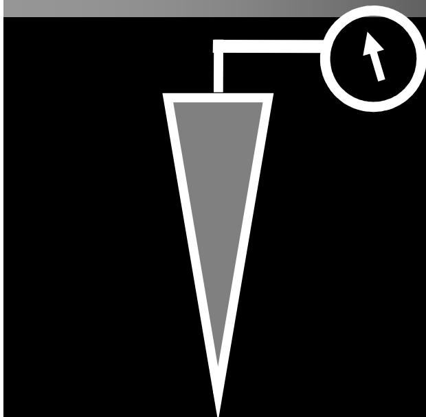
The STM measures the number of electrons that tunnel across the Vacuum barrier (tunnel current) at a fixed real space position
