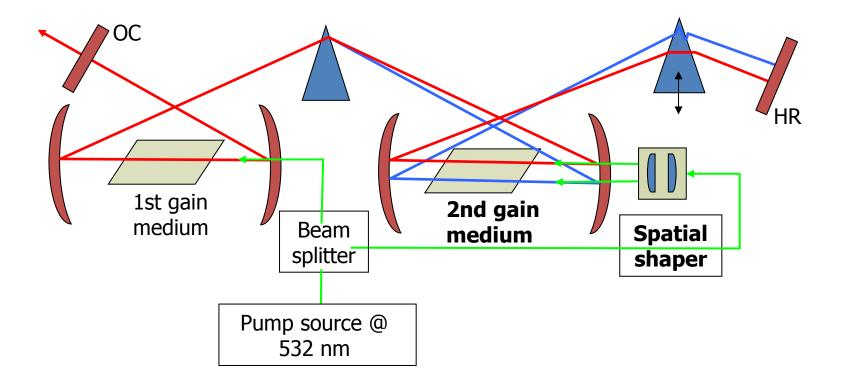
**Spatial** shape of pump = **Spectral** shape of gain
