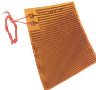
Kapton (polyimide film) heater Excellent radiation resistance
