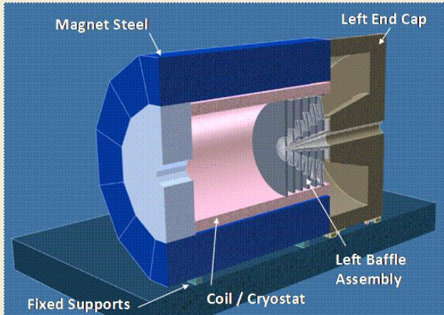
Proposed design provides sufficient acceptance, resolution, and shielding for broad PVDIS program
