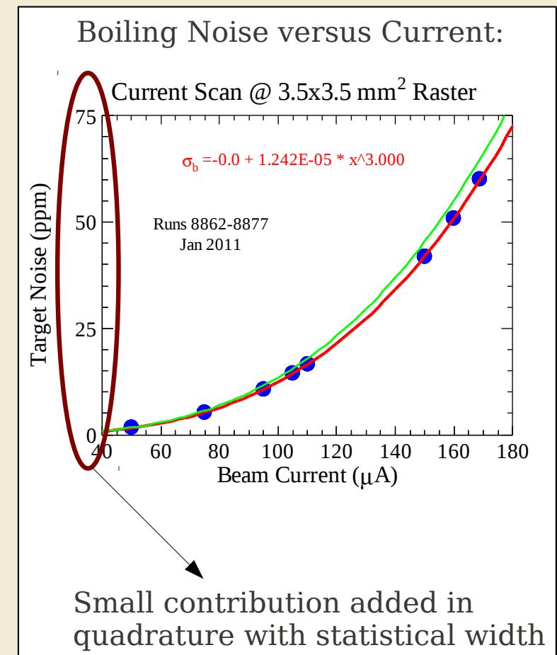
Boiling <60ppm = about 4% excess noise
