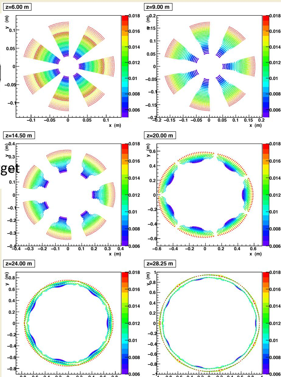
Radial Fields (edge effect) creates azimuthal defocussing which populates the full ring at the detector
