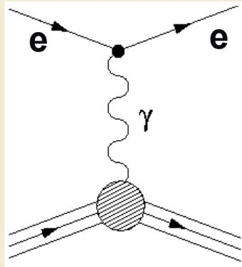
Electron scattering is (mostly) electromagnetic scattering.
