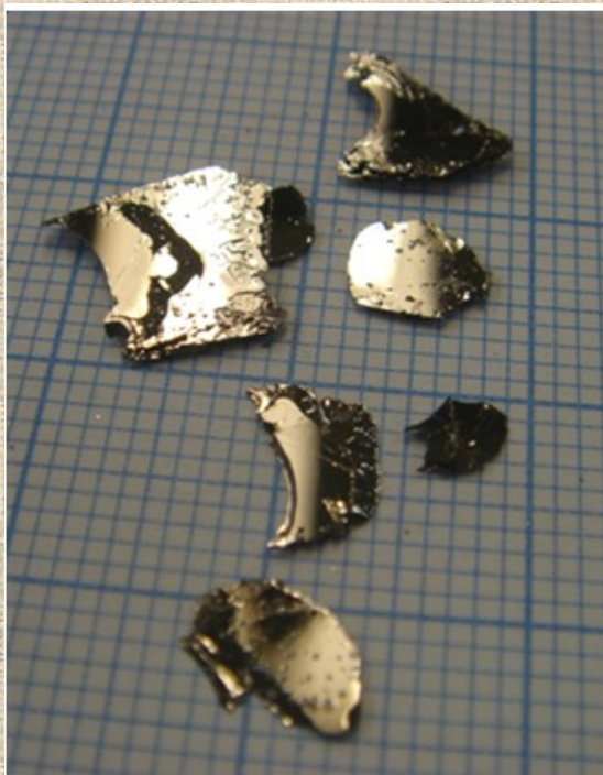
Crystals with \text{ThCr}_2\text{Si}_2 Structure ( \text{BaFe}_{1.84}\text{Co}_{0.16}\text{As}_2 )
