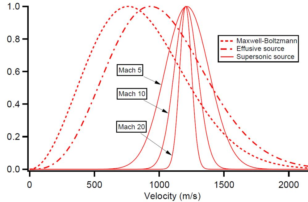
Figure 2.1: A comparison of the Maxwell-Boltzmann, effusive, and supersonic distribution functions for a sodium source with reservoir temperature of 800 K. Mach numbers of 5, 10, and 20 are used for the supersonic distributions.
