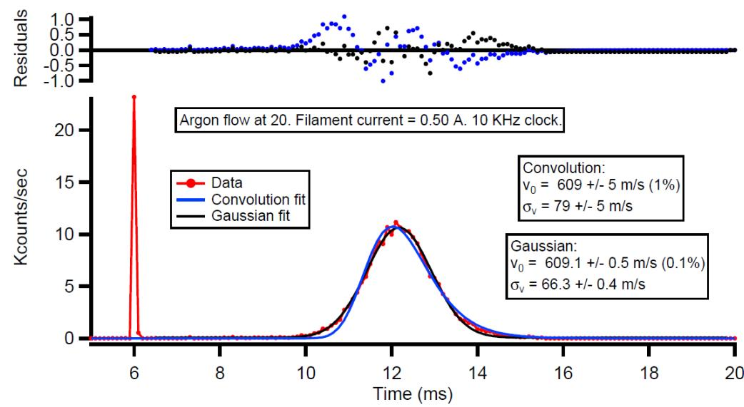
Figure 2.8: TOF measurement for a metastable argon beam. Two fits are made to the data: A Gaussian fit in black and a convolution of Equation 2.25 with a 0.35 ms impulse and metastable lifetime decay function in blue. The corresponding velocity distribution results are shown in the boxes.
