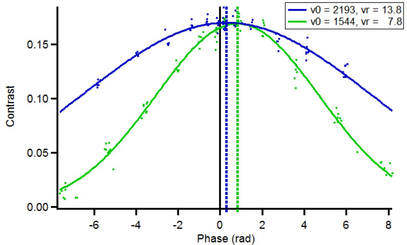
Figure 3.1: Two sets of raw contrast vs. phase data with different beam conditions and Gaussian fits.  $\Phi_{Cmax}$  is denoted by the dotted vertical lines. The larger  $v_0$  leads to a smaller  $\Phi_{Cmax}$ . Larger  $v_r$  leads to slower loss of contrast.
