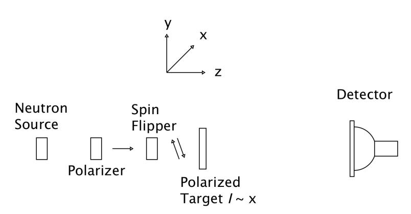
Ideally, the spin is along y such that  $\sigma.lxk$  is maximal and  $\sigma.k$  is zero.  $\sigma$  is shown making a small angle,  $+/-\theta$ , in the y-z plane. Because  $\sigma.k$  is non-zero there is a PV asymmetry  $\sim Sin(\theta)$ .
