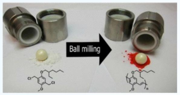
Ten minutes of processing in a ball mill polymerizes a white monomer (left) into a bright red conducting polymer, poly(2-methoxy-5-2´-ethylhexyloxy phenylene vinylene) (right). Credit: ACS Macro Lett. http://cen.acs.org/articles/92/web/2014/03/Ball-Mill-Grinds-Monomers-Polymer.htm
