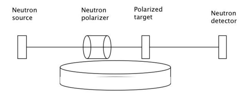
Rotate table that supports apparatus by 180 degrees and change the sign of all classical fields, B and J.
