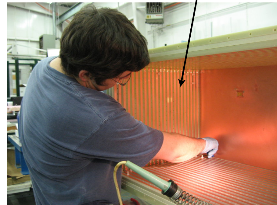
TPC Field Cage formed out of copper-clad G10 boards
