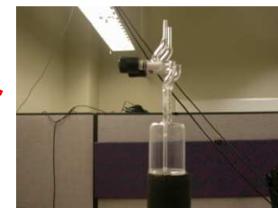
1 mCi ^{22}\text{Na} Radiation source with two gamma lines 511 and 1275 keV Placed inside massive lead collimator R_{\text{hole}} = 2.5\text{mm} L_{\text{hole}} = 8.5\text{cm}
