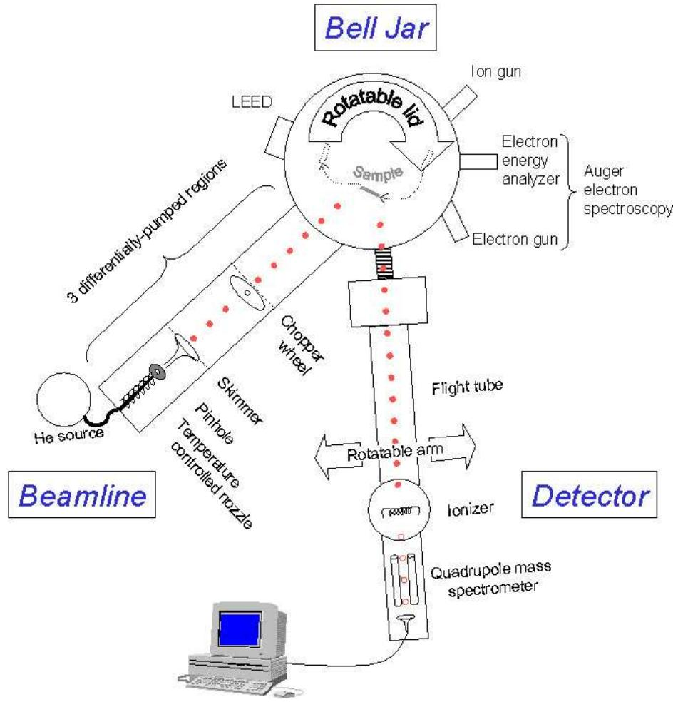
Molecular Beam-Surface Scattering Apparatus
