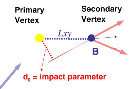
Silicon Vertex Trigger (SVT) – part of trigger system that finds displaced tracks and triggers on heavy hadrons
