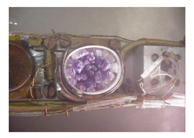
A photo of the target cell after the beam exposure. The beads in the center turned purple from the exposure while the beads at the edges did not receive much beam. Size: 1-2 mm
