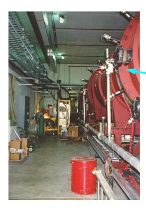
at z = 90 m, the two beams enter the KTeV decay region, which is an evacuated volume held at ~1 µTorr and is 69 meters in length.
