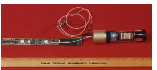
affixed to each crystal was a photomultiplier (PMT) with a DPMT (digital PMT) board. The DPMT board was created to digitize and buffer the anode signal from the PMT's.
